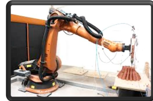
Large-Scale Rapid Prototyping Robots: Industrial Robot Arm Extruders and Building-Scale 3D Printers from: http://www.hizook.com
